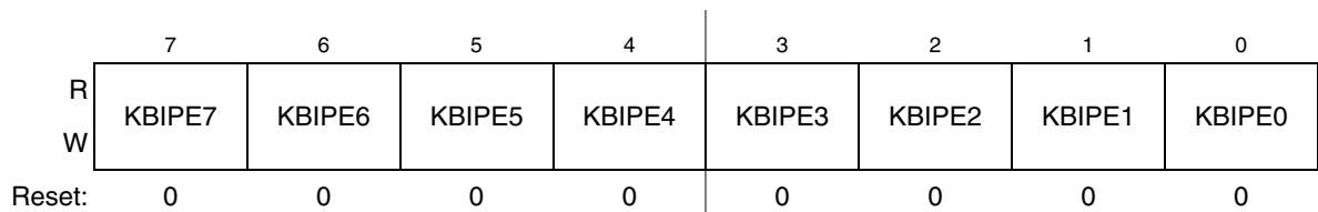
Figure 9-4. KBI Pin Enable Register
