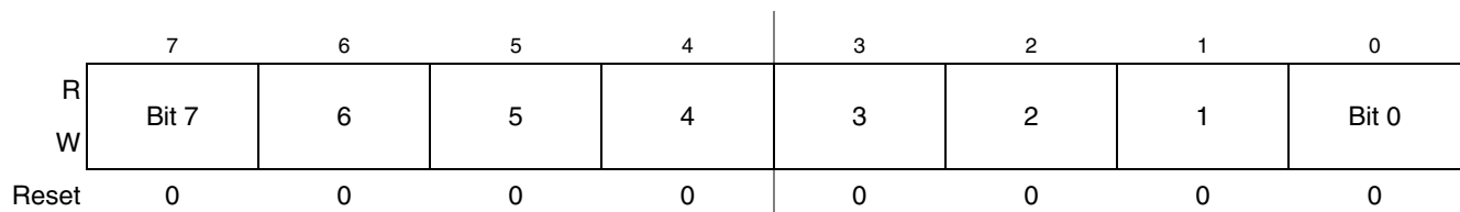
Figure 15-10. SPI Data Register Low (SPIxDL)
